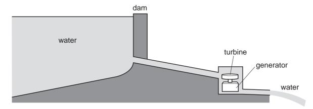
The water flows to a turbine and turns a generator.
