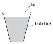
When the lid is removed, the rate of heat loss from the drink increases.
